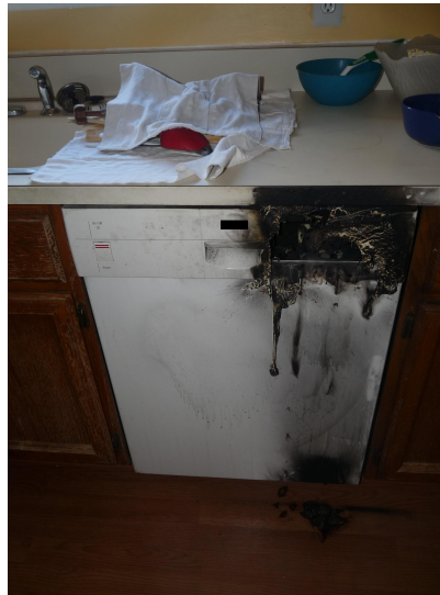
Failure of dishwasher controls
